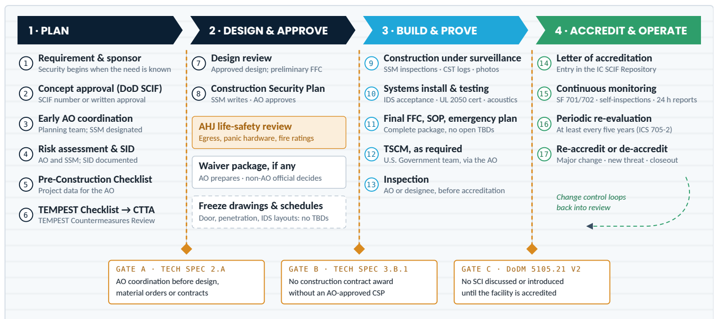
Figure 4.1 · The lifecycle in four phases and seventeen steps. Steps 3 through 8 normally precede contract award; CSP approval always does. Exact submittals and sequence vary by agency; your AO sets them.
